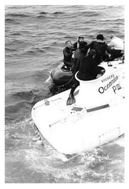
submarine onto the ship snapped. When the cable broke it also removed a rear hatch on Pisces Ill that allowed water to enter a watertight sphere and sink Pisces.
